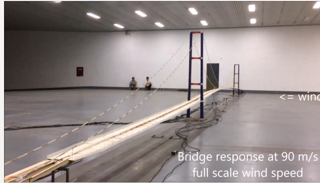
1:190 scale full bridge wind tunnel model
